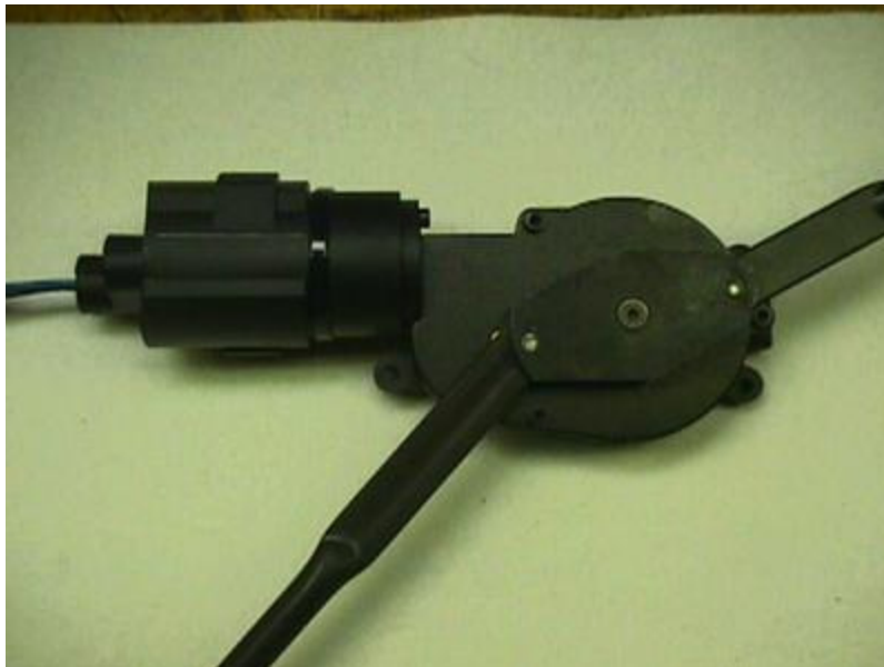
Motor and gear box, crank plate side
