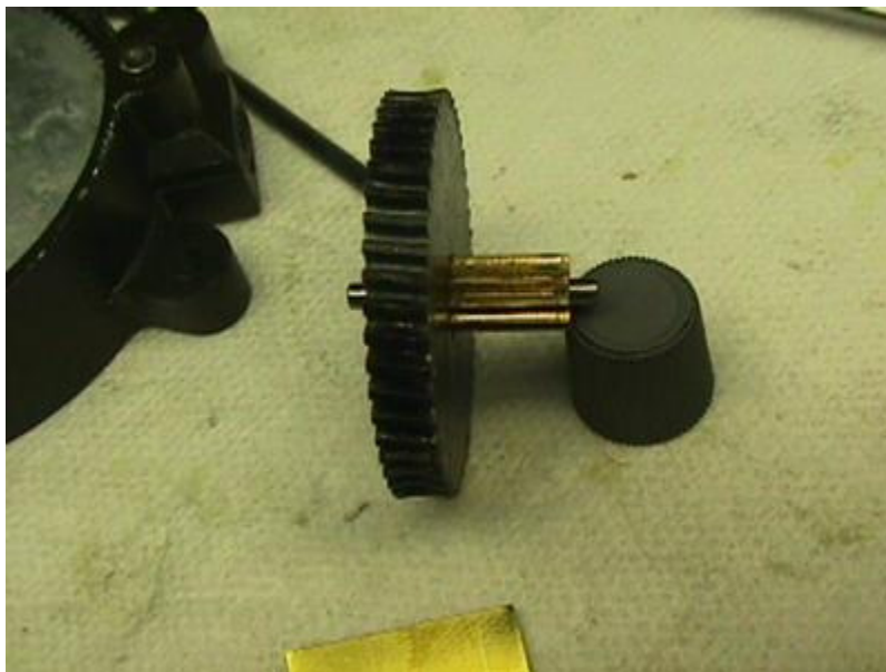
Fibre worm wheel and brass pinion
