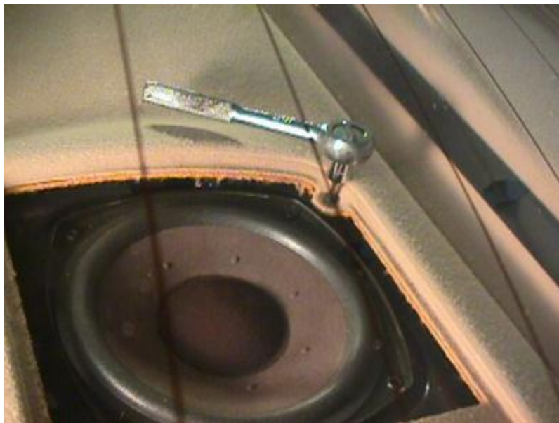
Removing the torx speaker screws
