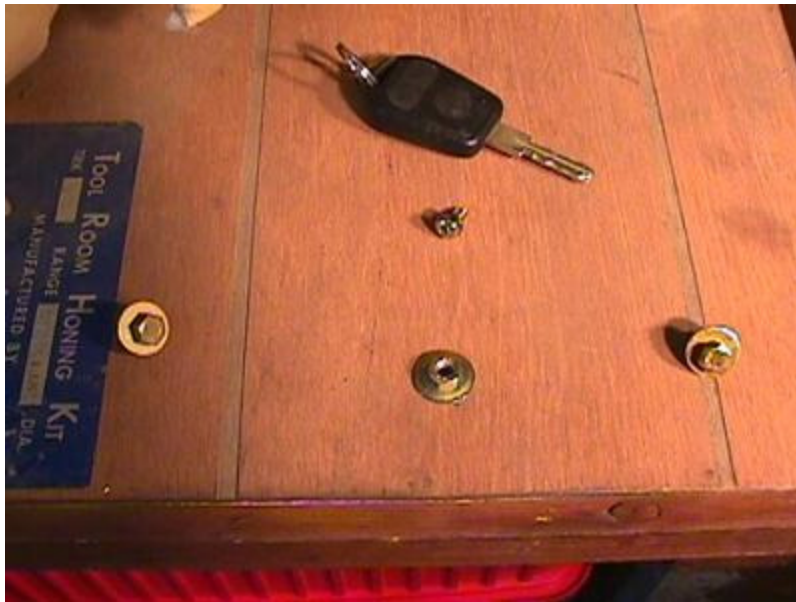
Trunk roof fasteners for the sun screen shelf
