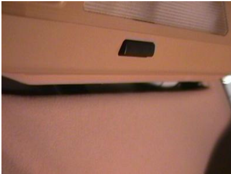
Lift out the lamp housing
