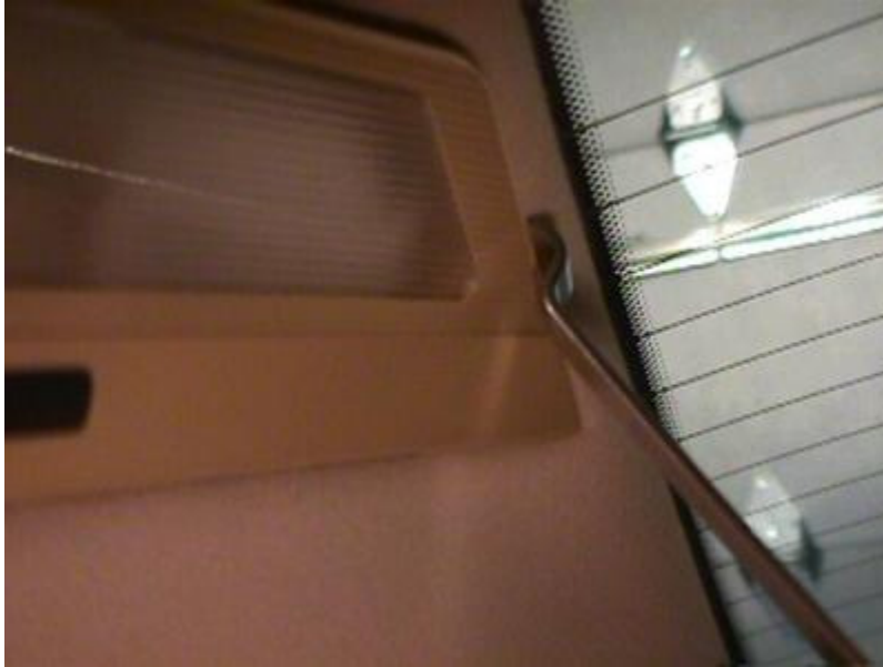
Free the back of the lamp housing
