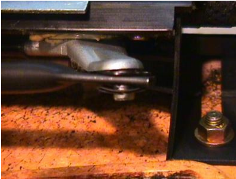
Spring clip holding a crank pin
