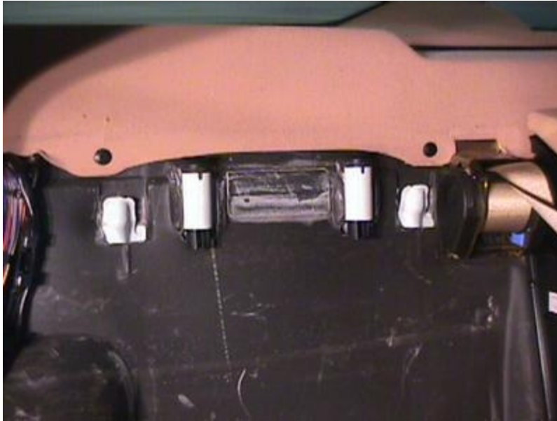
Speaker trim panel pop fasteners in place
