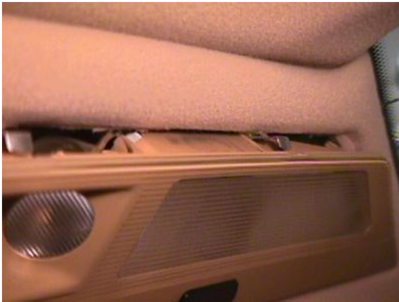
Free the top edge of the lamp housing
