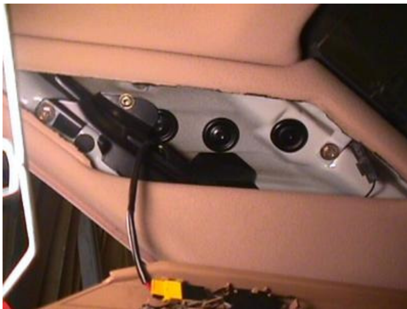
Three bolts hold the pillar cover
