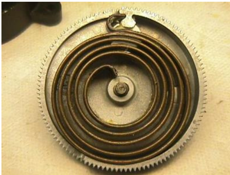
Main spring installed
